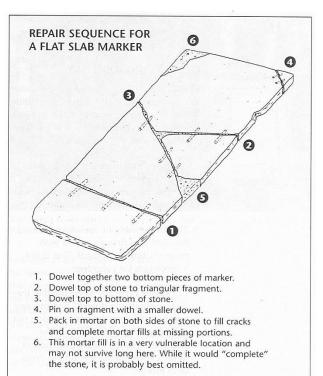
described above. Large pip clamps and nylon belts that can be tensioned are useful for holding large stones together. Use wood spacers to protect the edges of the marker.
