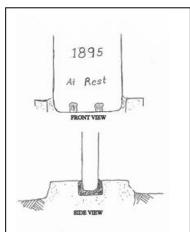
Bed headstone on lead shims. Use lead wedged on each side to keep headstone verticaly aligned. Pack in mortar and finiah with slightly sloped mortar pointing. Do no feather mortar on the top of the base.
