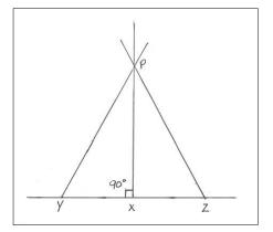
Figure 1 Construction of the Perpendicular. X = the point from which a 90 ° offset is required Y,Z = points equidistant from X on a straight line. P = a point at which two measuring tapes attached to Y and Z cross the same length.
