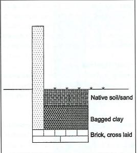
The drawing shows the cross section of a repair when clay bricks are used as a base and bagged clay is used to strengthen the repair.
