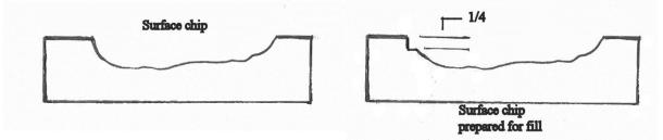
Chips and breaks need to be prepared as shown in this illustration. A feathered edge repair is prone to failure.
